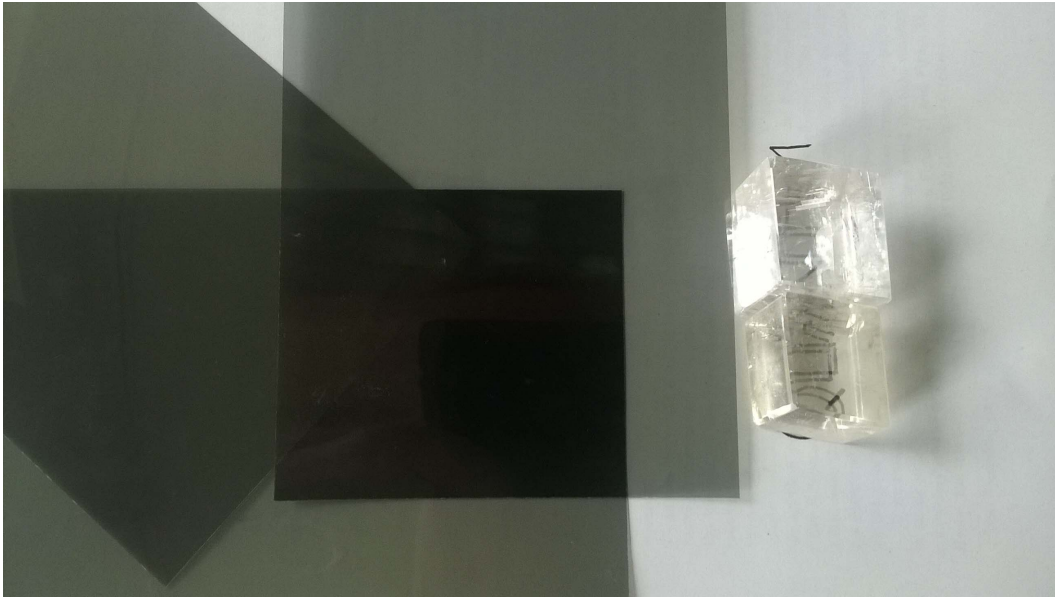
Figure 12: My experimental set-up costs about 90 Euros. The left half shows four polaroid filters, and on the right half there are two calcite crystals. The following experiments can be performed easily with these optical elements.
